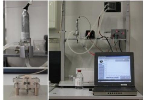
Characterization system for QCM sensors on liquid environments under static and dynamic conditions (biosensors).
