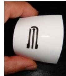
On wafer characterization system and inkjet printing setup with deposition examples (SAW devices, resistive sensors, flexible contacts).
